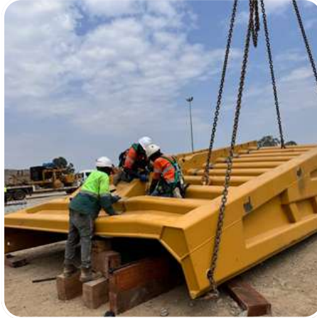
Dump Truck CAT777E Trays Assembly : Barrick North Mara Mine
