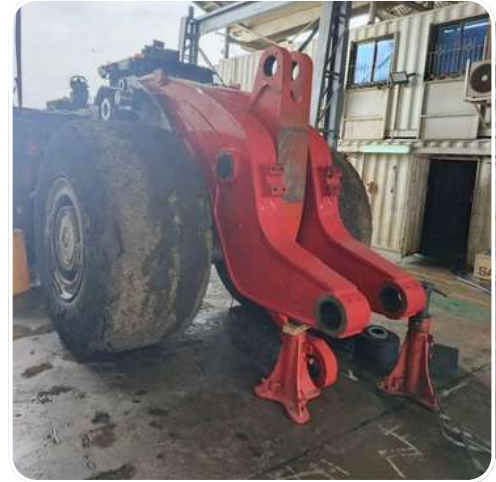
UG Loader H-Frame Refurbishment: Barrick North Mara Mine
