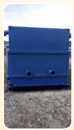
Converting Containers to Water Tanks for North Mara Underground
