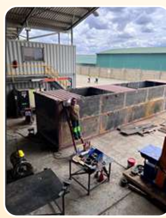
Converting Containers to Water Tanks for North Mara Underground
