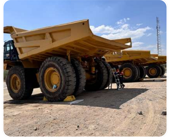
Dump Truck CAT777E Trays Assembly : Barrick North Mara Mine
